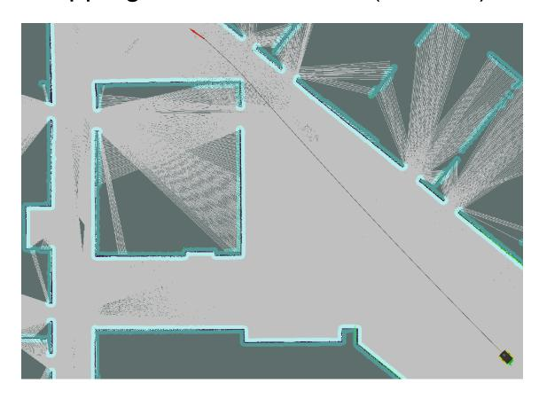
A Lidar Based Map of the Delta 3rd floor building
